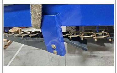
Install the mounting plate for the roller jack.
