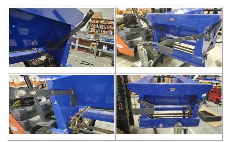
Find this bracket and mount it close to the end on top onto the brackets on the top of he frame.
