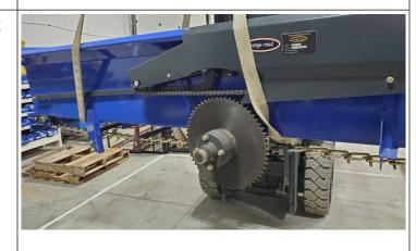
Take out the bolts from the hub and install the wheels. Torque the bolts to 35 ft  $\cdot$  lbf . Fill up the air to 29 PSI.
