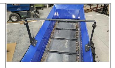
Find this bracket and mount it at the end as guard for the spreader paddles.
